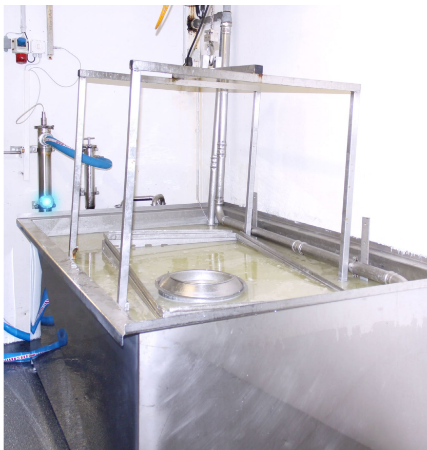
The AQD-ST reliably sterilises the brine despite its high turbidity and allows the cheesemaker to control the flora in the brine.
